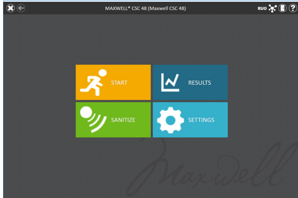
Figure 42. 'Home' screen. Selecting the Sanitize button begins the process for UV treatment of the Maxwell® CSC 48 Instrument.
