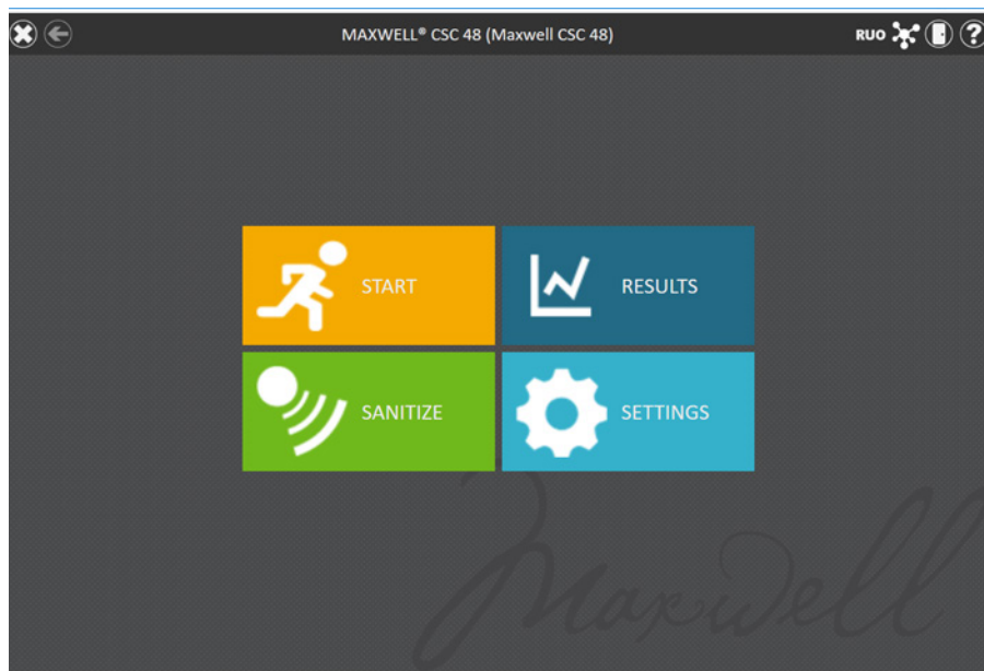
Figure 22. 'Home' screen. Selecting the Start button begins the process of running an extraction method on the Maxwell® CSC 48 Instrument.
