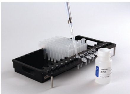
Figure 2. Setup and configuration of the deck tray. Elution Buffer is added to the elution tubes as shown. Plungers are in well #8 of the cartridge.
