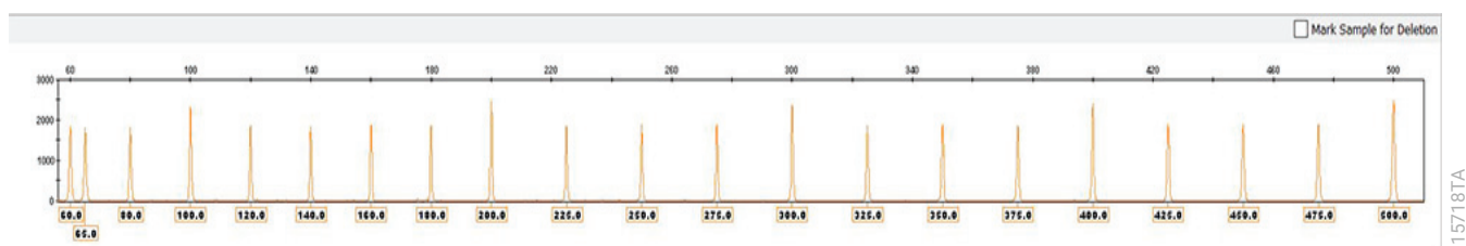
Figure 33. WEN Internal Lane Standard 500. An electropherogram showing the WEN Internal Lane Standard 500 fragments.
